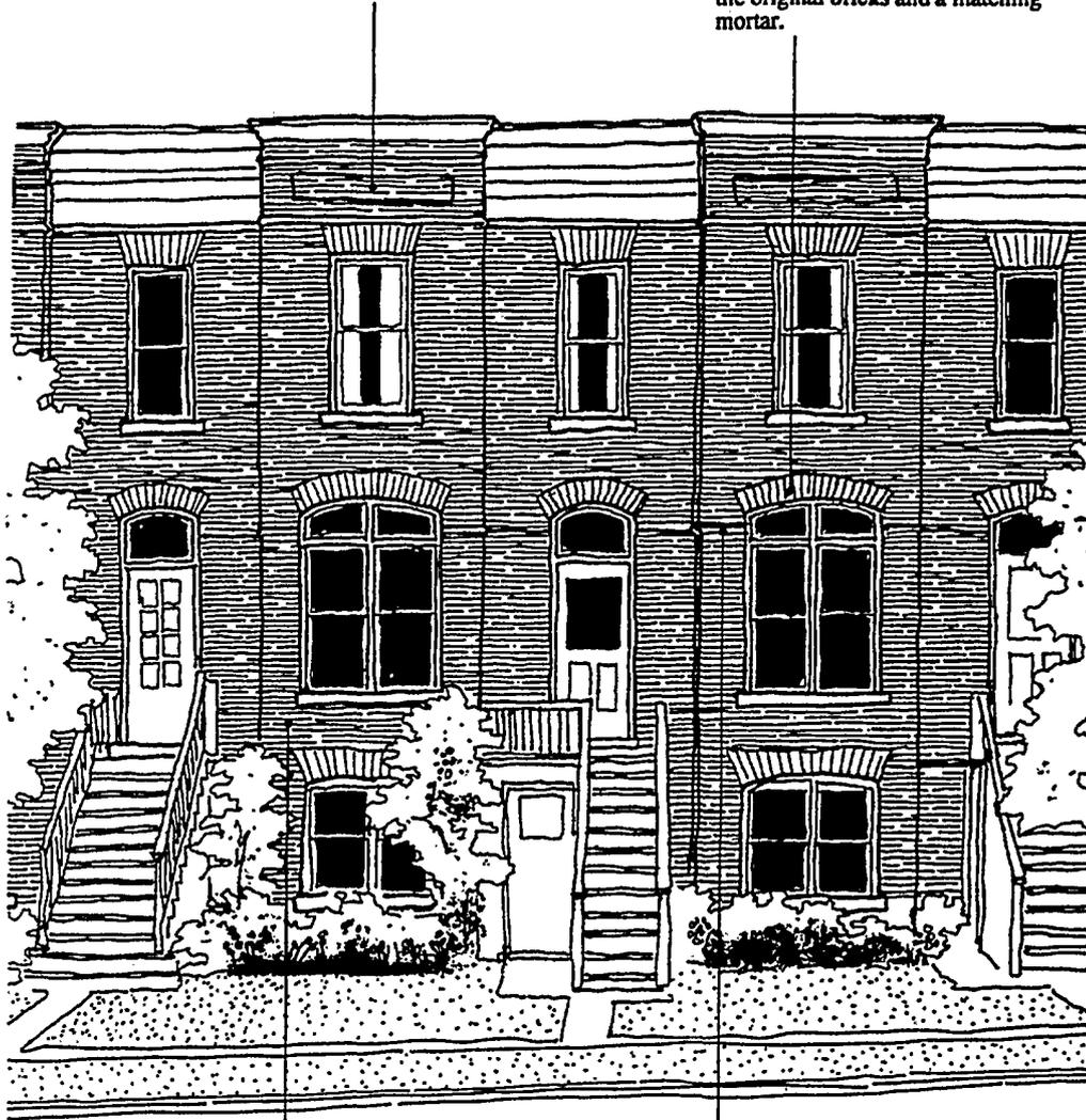
Dirt does not generally harm masonry. In fact, it provides character and age to a historic building. Only clean when absolutely necessary, and use the gentlest method. Never sandblast!
