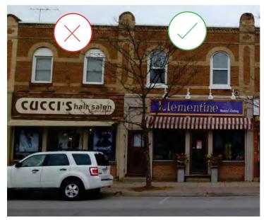
102. Original window openings and patterning have been maintained in new window design and installation at 19 Queen Street North (right) in contrast to poorly modified window openings on 23 Queen Street North (left), Bolton. (Source: ERA)
