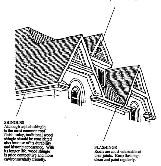
Roofs create the building silhouette, like those at 15 & 17 Hilda Place shown above. The roof finish contributes colour, texture and pattern. The finish naturally deteriorates and periodically needs replacement. The choice of finish should complement the building style. Wood shingle is the traditional and most attractive finish. Consider carefully the merits of different finishes. Initial price is not the only criterion. Longevity and character on an historic building are important too!
