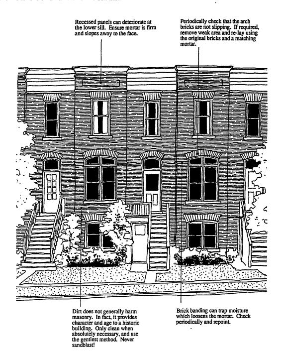
Brick is the predominent building material in the Area. In the circa 1889 Nelson Terrace on Courtland Avenue, the brick becomes a work of art, with arches, banding, recessed panels and projecting bays. Periodically repointed, brick can last indefinitely. Care should be taken when cleaning not to damage the brick face. Repointing should match the original mortar.
