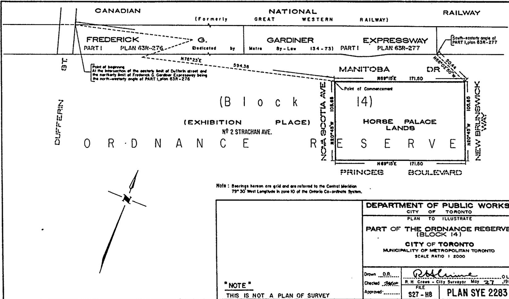
Note: Bearings hereon are grid and are referred to the Central Meridian 79° 30' West Longitude in zone 10 of the Ontario Co-ordinate System.
