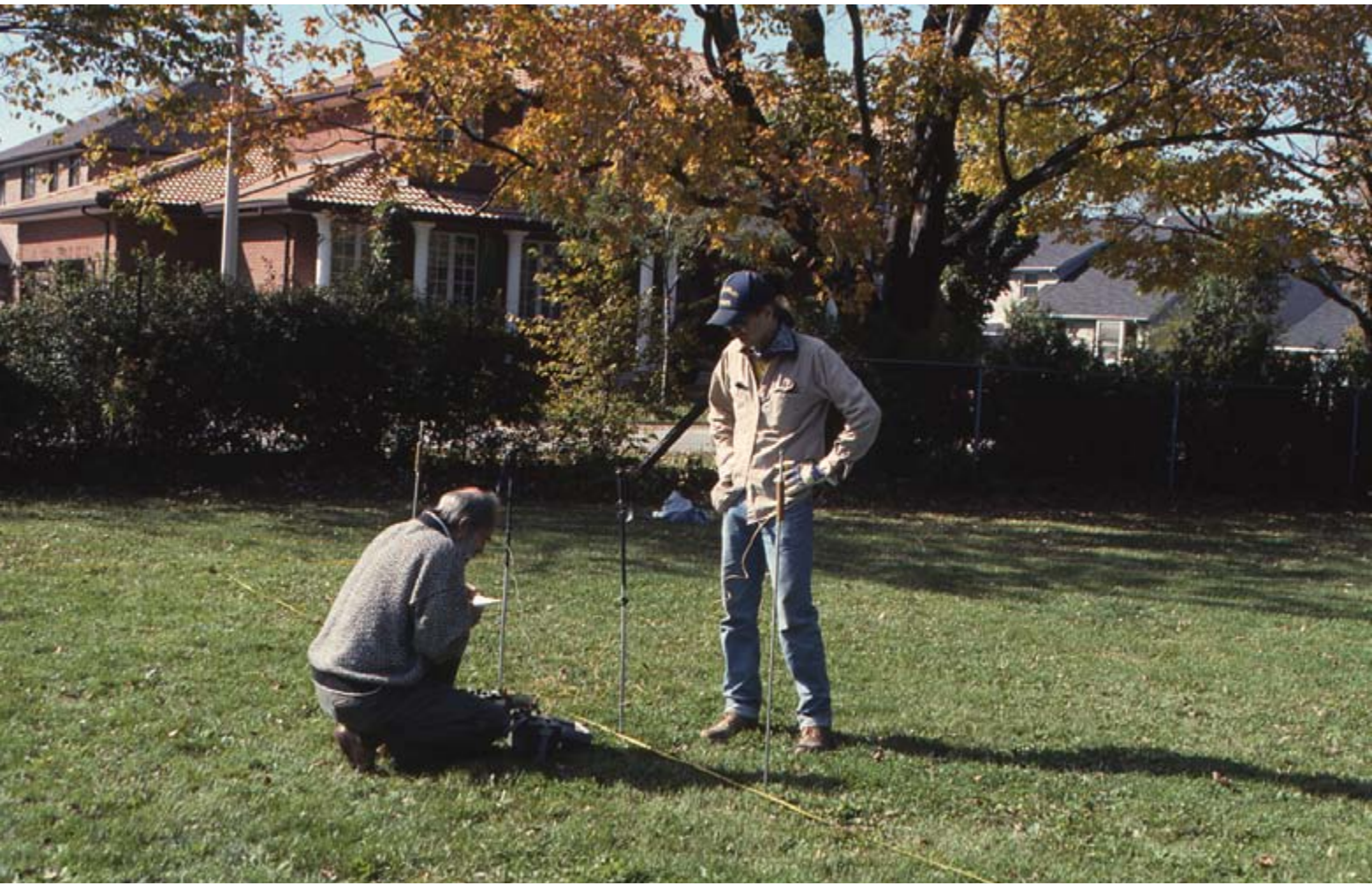
Several geophysical methods were used at the Trust's Chedoke Estate in Hamilton, including resistivity (shown in photo), magnetometer and electromagnetic survey
